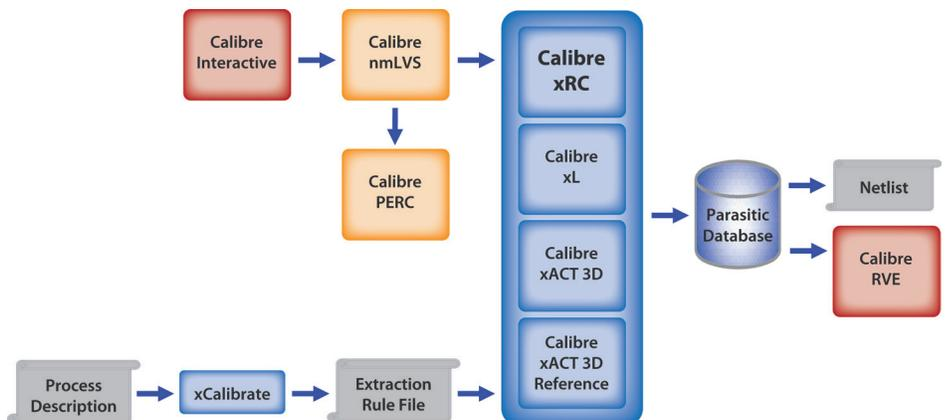
Calibre xRC is fully integrated into the Calibre verification suite for seamless creation of netlists and parasitic debugging in the design environment using Calibre RVE. xCalibrate is used by foundries to create extraction rule files, and the same rule files can be used by Calibre xRC, Calibre xL, Calibre xACT 3D and Calibre xACT 3D Reference.
