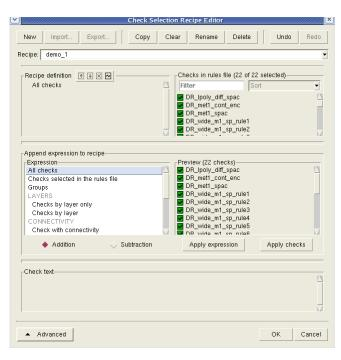
Check recipes are an effective way to repetitively run selected checks.
