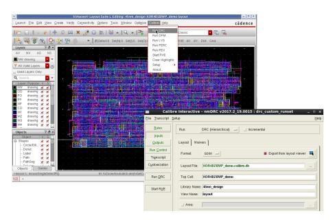
The Calibre Interactive interface is the invocation GUI for Calibre DRC, LVS, PERC, DFM and xRC/xACT tools for physical verification, circuit verification and parasitic extraction. It's easily accessed from the menu bar within most layout design environments. The Calibre Interactive GUI also gives users access to the Calibre RVE interface, the robust and easy-to-use results viewing environment.
