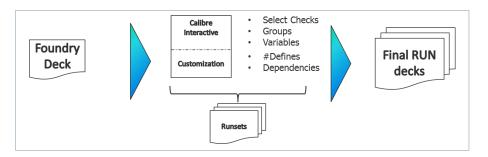
Runsets simplify set-up and ensure consistency.
