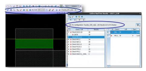
Designers can highlight results using either the Calibre RealTime Custom toolbar or the Calibre RealTime Custom results window.
