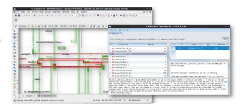
Designers can highlight results using either the Calibre RealTime toolbar or the Calibre RealTime-RVE window.
