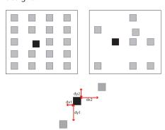
Optical grid/pitch checking uses sophisticated algorithms to assess placement for lithographic sensitivity.
